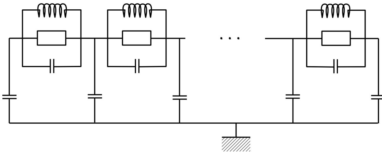
$$Y_{n-1/2}(V_n - V_{n-1}) + Y_{n+1/2}(V_n - V_{n+1}) - i\omega C_n^g V_n = 0 \quad \text{linear "wave" equation}$$
